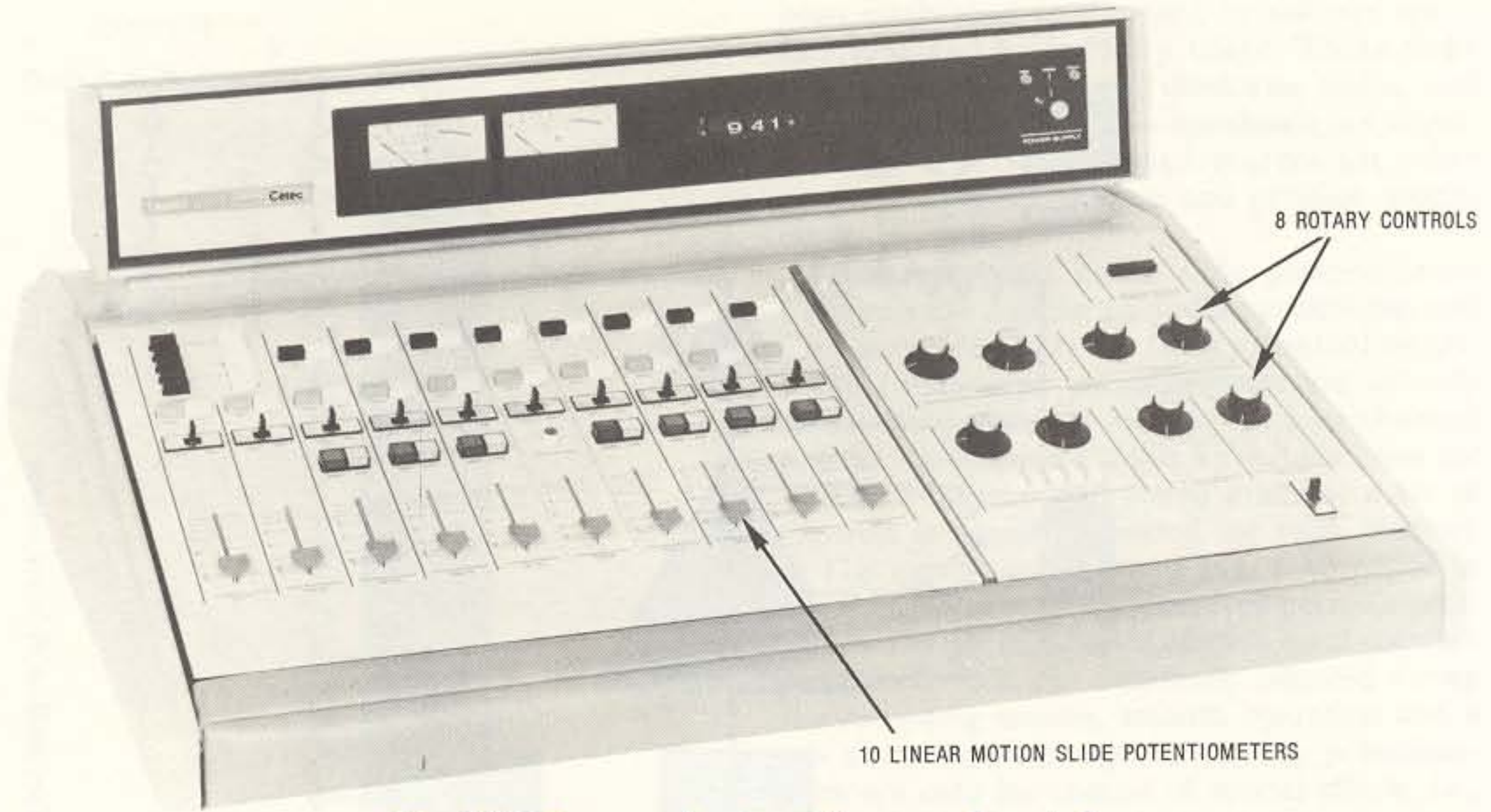
Fig. 5-10 Master mixer board for recording studio (Cetec, Inc.)
