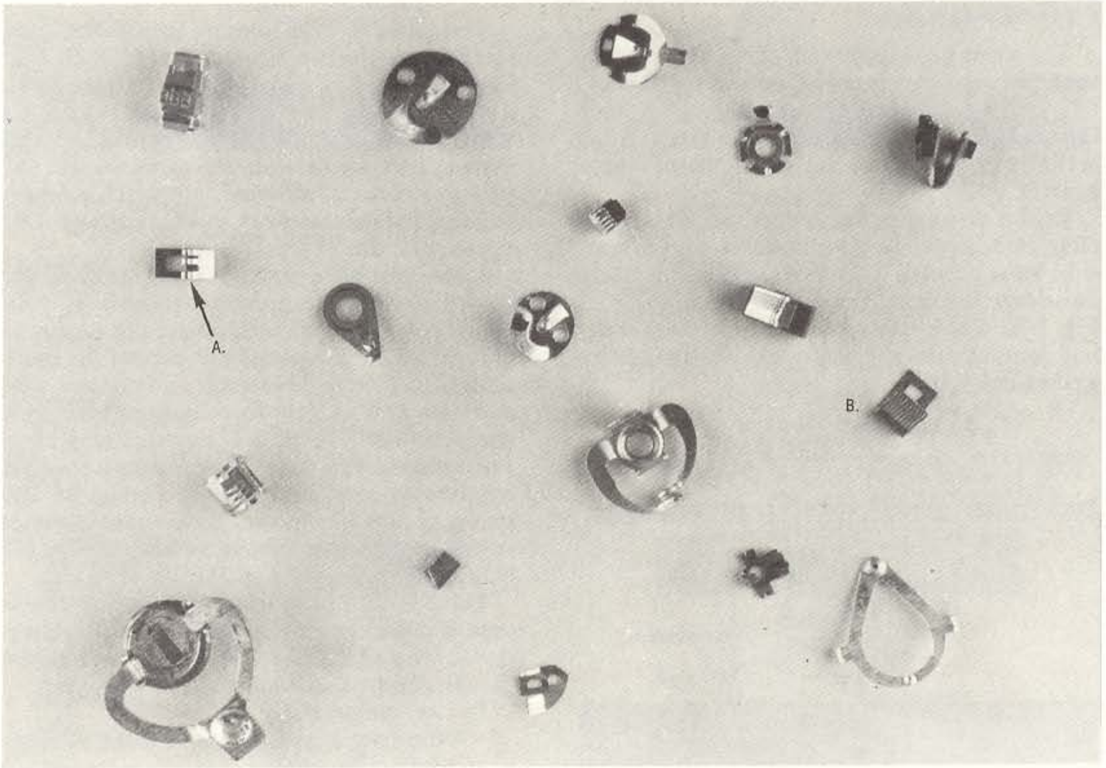
Fig. 7-24 Moveable contacts come in many different forms
