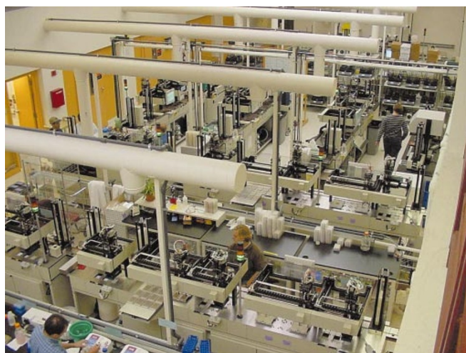
Figure 3 The automated production line for sample preparation at the Whitehead Institute, Center for Genome Research. The system consists of custom-designed factory-style conveyor belt robots that perform all functions from purifying DNA from bacterial cultures through setting up and purifying sequencing reactions.
