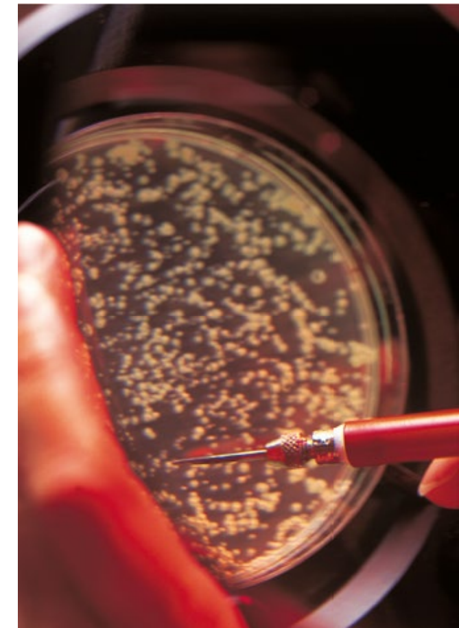
The number of bacteria colonies growing on test culture mediums is a measure for the effect of disinfectants
