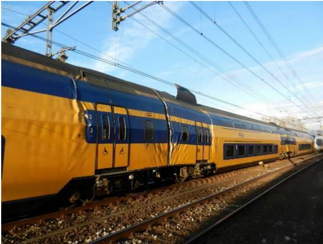
Fig. 3: The buckling action of the coaches of the VIRM-type intercity absorbed much kinetic energy. Picture by W.R. Beukenkamp
