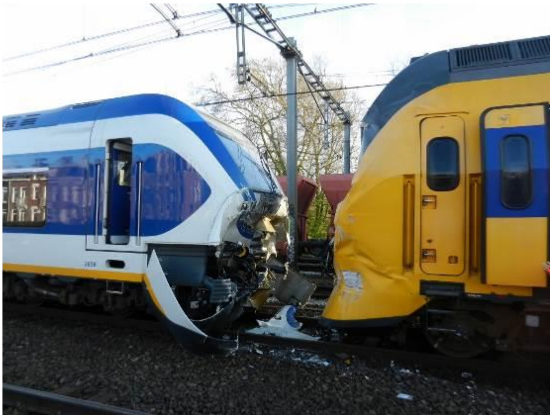
Fig. 4: The front of the SLT type Sprinter. The crash buffers have been pushed aside by the front of the VIRM type intercity. Picture by W.R. Beukenkamp
