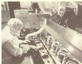
Disctronics' Melbourne CD plant - although fully automated, the top-coating process is subjected to constant visual checking.
