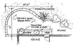
Remember that the area needs to have gradient or slope, so water can run off the pavers to prevent pooling or ponding that can damage the pavement over the long term.
