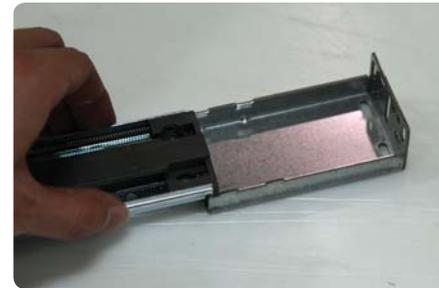
Temporarily place the back of the large drawer box slide into the mounting bracket.
