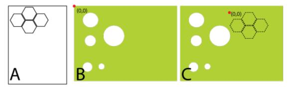
In the figure, A is the pattern to cut, B is the piece of material with the Home Position in the upperleft corner and C shows the Home point moved to a position where the pattern can be cut without issues.
