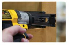
Place the slide into the bracket, and attach the final screw (A) through the frame. Tip: Pull the slide forward slightly to expose the hole.
