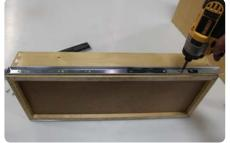
Locate the small drawer box slide, and using two screws (A), fasten it to the drawer box as shown.
