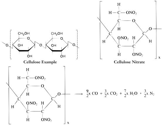
Reaction of the Cellulose Nitrate to form the following products.
