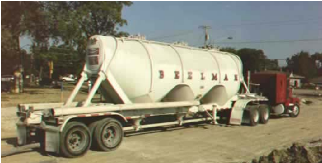
Figure 5: Example of tanker trucks typically used for dry lime delivery
