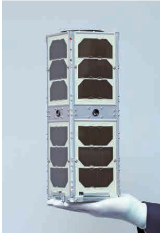
The further miniaturized CE-SAT-III measures 100 mm x 100 mm x 300 mm
