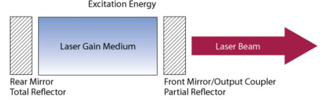
Fig. 1. The component parts of a typical laser
