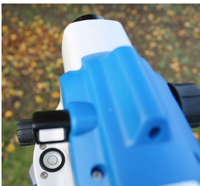
The levelling bubble should be central
