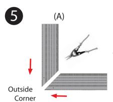
For outside corners (A) or inside corners (B), mitre cut both adjoining sections. Notch the front edge of one section to create an overlap.
