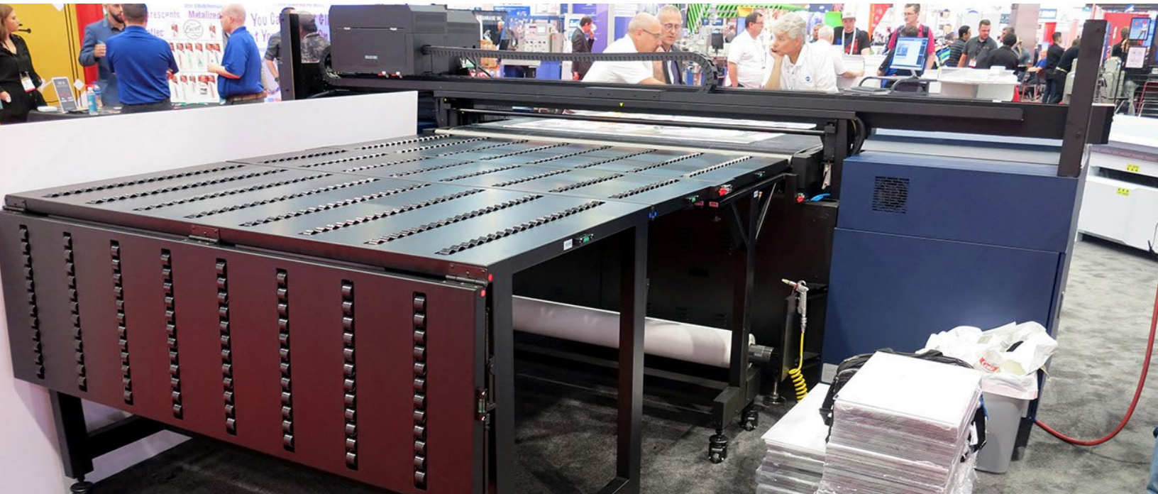
Rear and front view of the Konica Minolta AccurioWide 160 UV-curing combo printer. These models come with LED UV-curing lamps.
