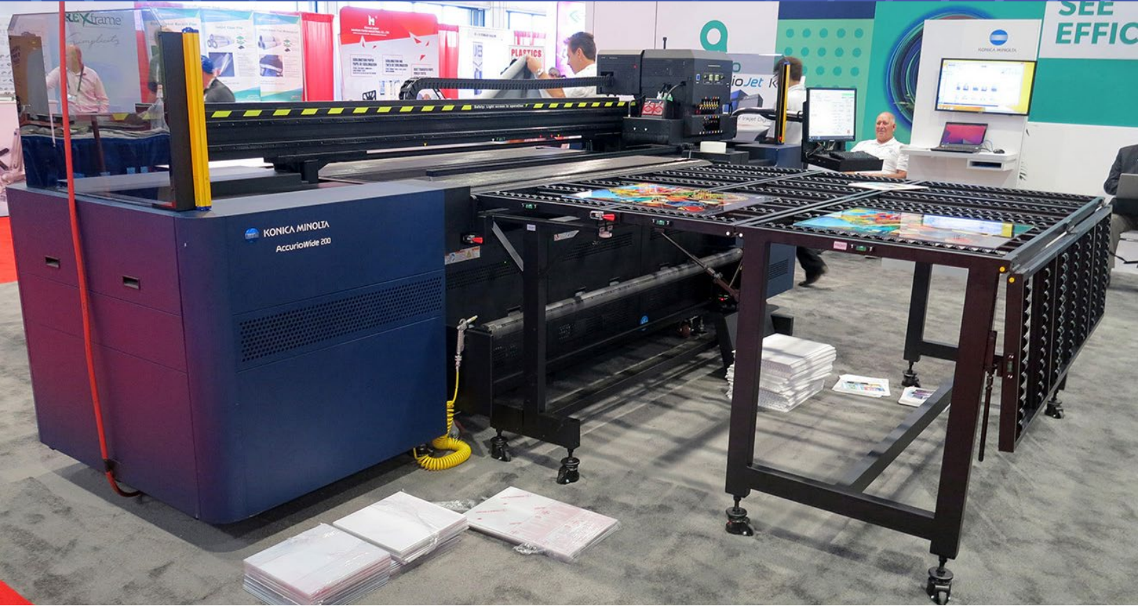
Put on the tables and you can print thick flat materials. This is the Konica Minolta AccurioWide 200.
