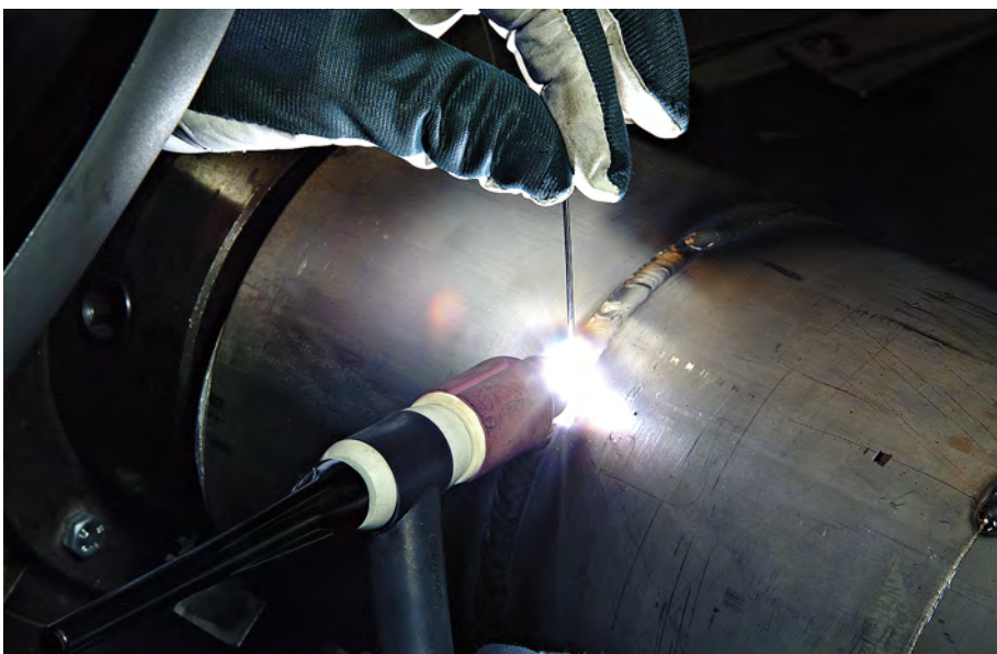
Gas tungsten arc welding. © Sandvik
