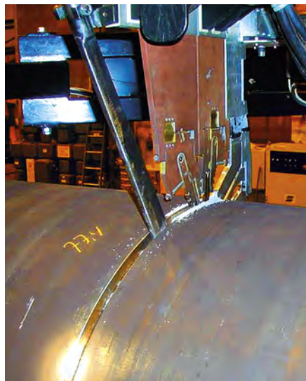
Submerged arc welding. © Outokumpu
