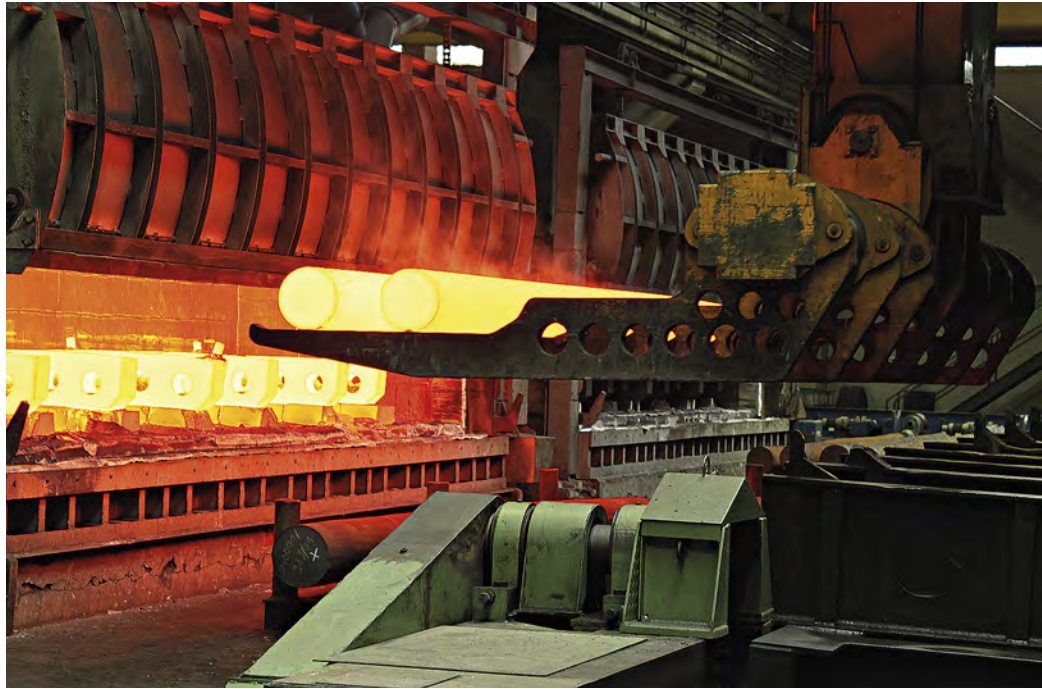
Hot duplex stainless steel is removed from the heat treating furnace after solution annealing. © Bosch-Gotthard-Hütte
