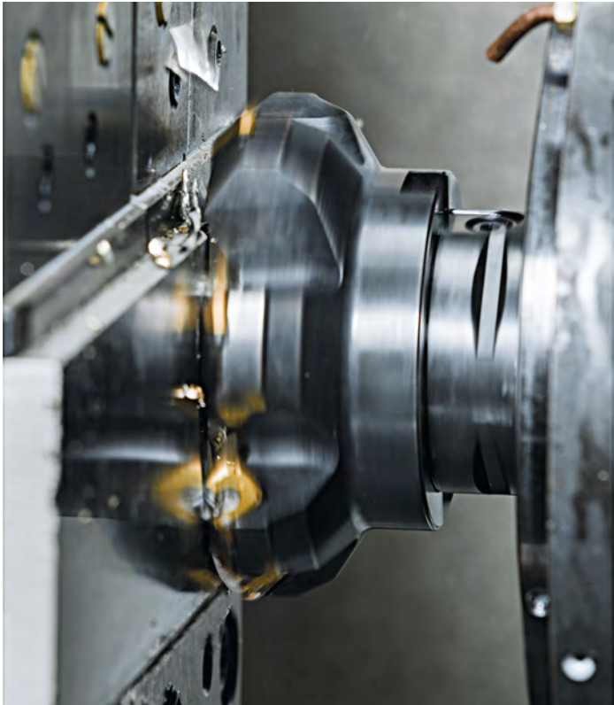
Face milling operation. © AB Sandvik Coromant
