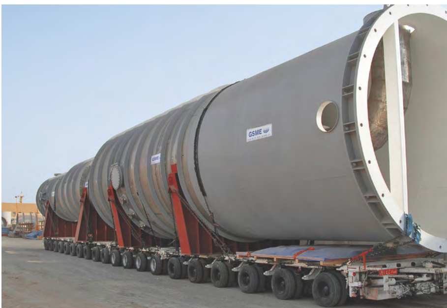
2507 stainless steel falling film evaporator. © Gary Carinci, TMR Stainless
