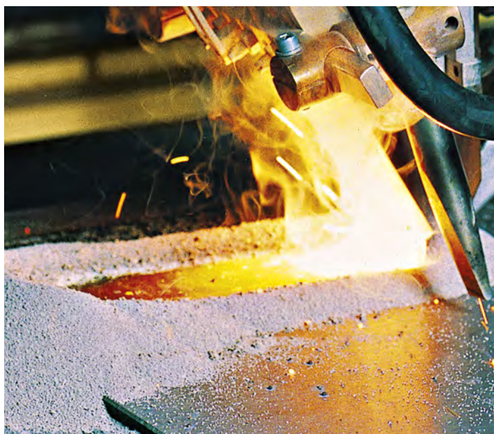
Electro-slag weld strip overlay. © Sandvik
