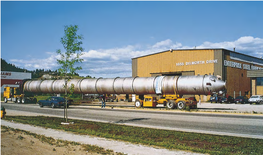
2205 oxygen delignification reactor, Enterprise Steel Fab, Kalowna, Prince George, British Columbia, Canada. © Outokumpu
