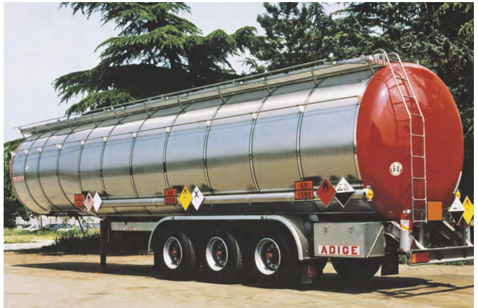
Lean duplex stainless steel asphalt hauling tanker. © Outokumpu
