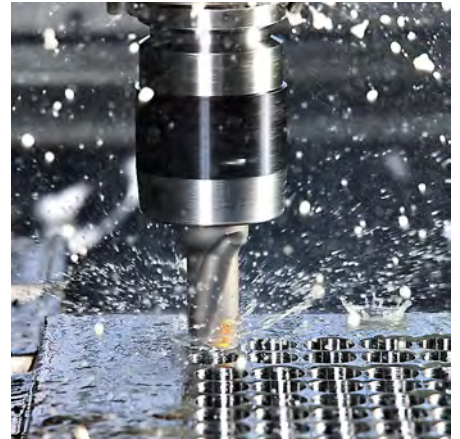
Twist drilling operation. © Sandvik
