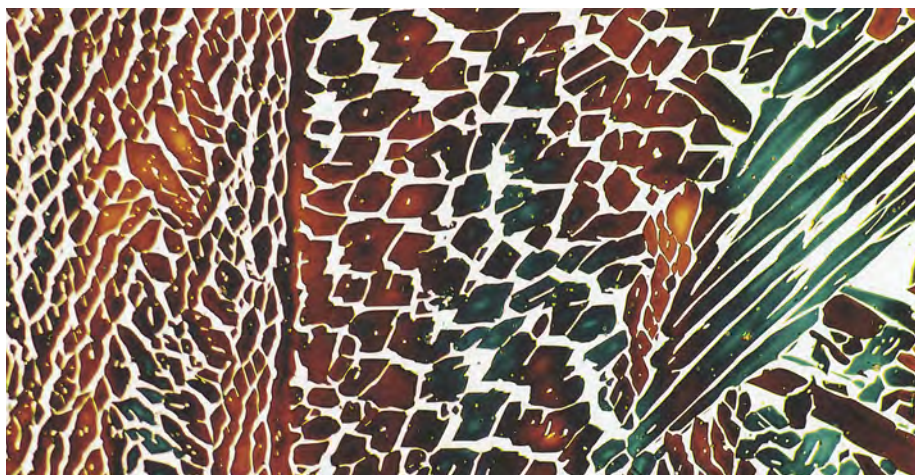
Metallographic structure of 2205 duplex weld metal, 500x. © Lincoln Smitweld bv
