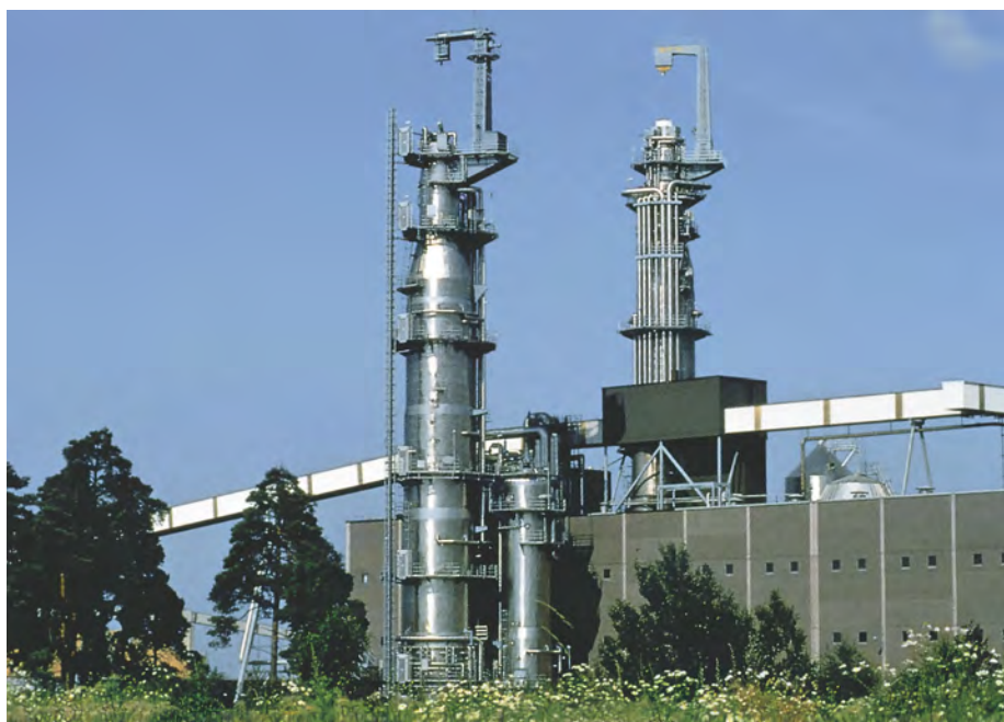
2205 continuous sulphate pulp digester and impregnation tower, Sodra Cell Mönsteras, Sweden. © Kvaerner Pulping
