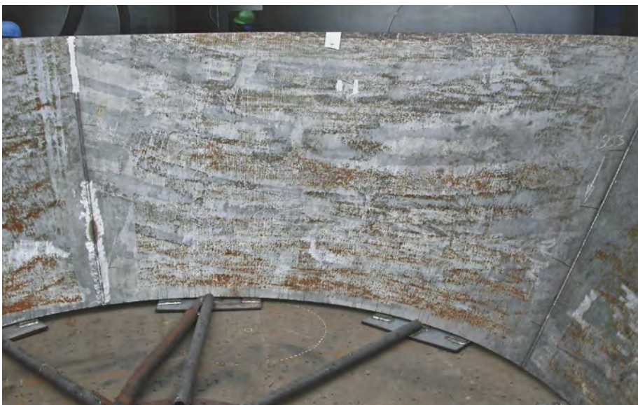
Embedded iron in roll formed duplex stainless steel plate fabrication. © Gary Carinci, TMR Stainless
