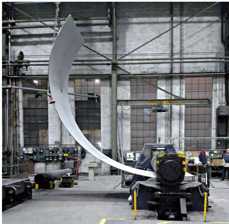
Roller bending of 28 mm thick duplex stainless steel plate. © Outokumpu
