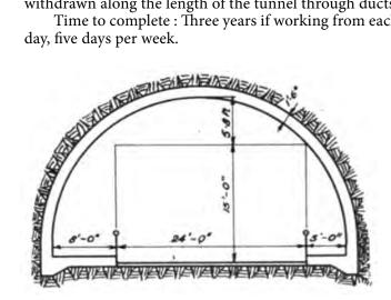
Diagram of a section of the road tunnel showing cycle and footway on the left, the roadway centre, and cycleway on right.
