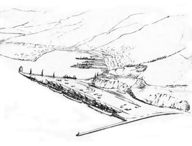
Part of the £3,500,00 Harbour enlargement project, which involves the reclamation of 41 acres of land, and the construction of some 2000 feet of additional deep-water berthage.
