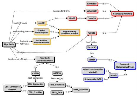
Figure 5. The geometric representation for the rigid bodies model
