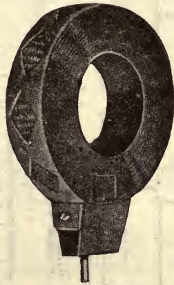
FIG. 27. — A typical plug-in "honeycomb" tuning coil.
