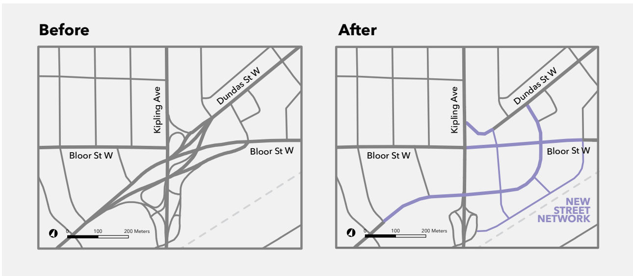
Figure 29: Street network before and after pedestrian-friendly redesign
