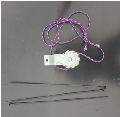
Fig. 23: Zip ties, tensioner, and parachute cord used for attaching plastic. Photo: K. Orde
