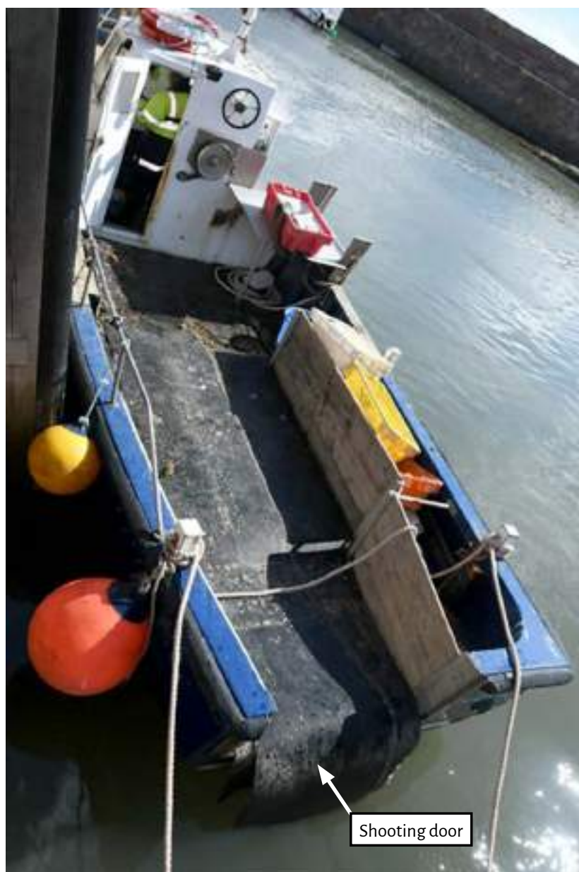
Figure 2: The shooting door (drop-in closing board removed)
