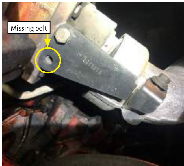
Figure 4: Fractured bracket and missing bolt
