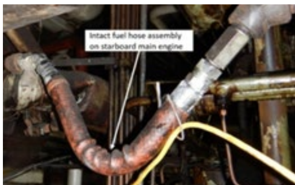
Flexible fuel hose assembly on the inboard side of the starboard main engine (Photo credit: TSB)
