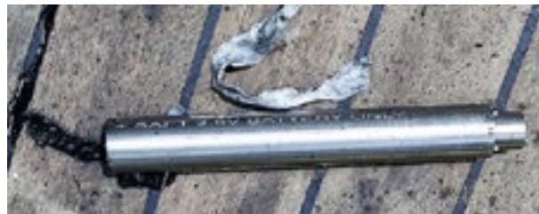
Figure 1: Damaged battery tube
