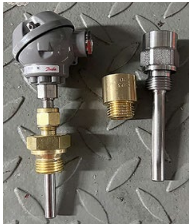
Figure 3: The new temperature probe fitting
