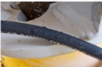
Incompatible hydraulic hose blistered during use
