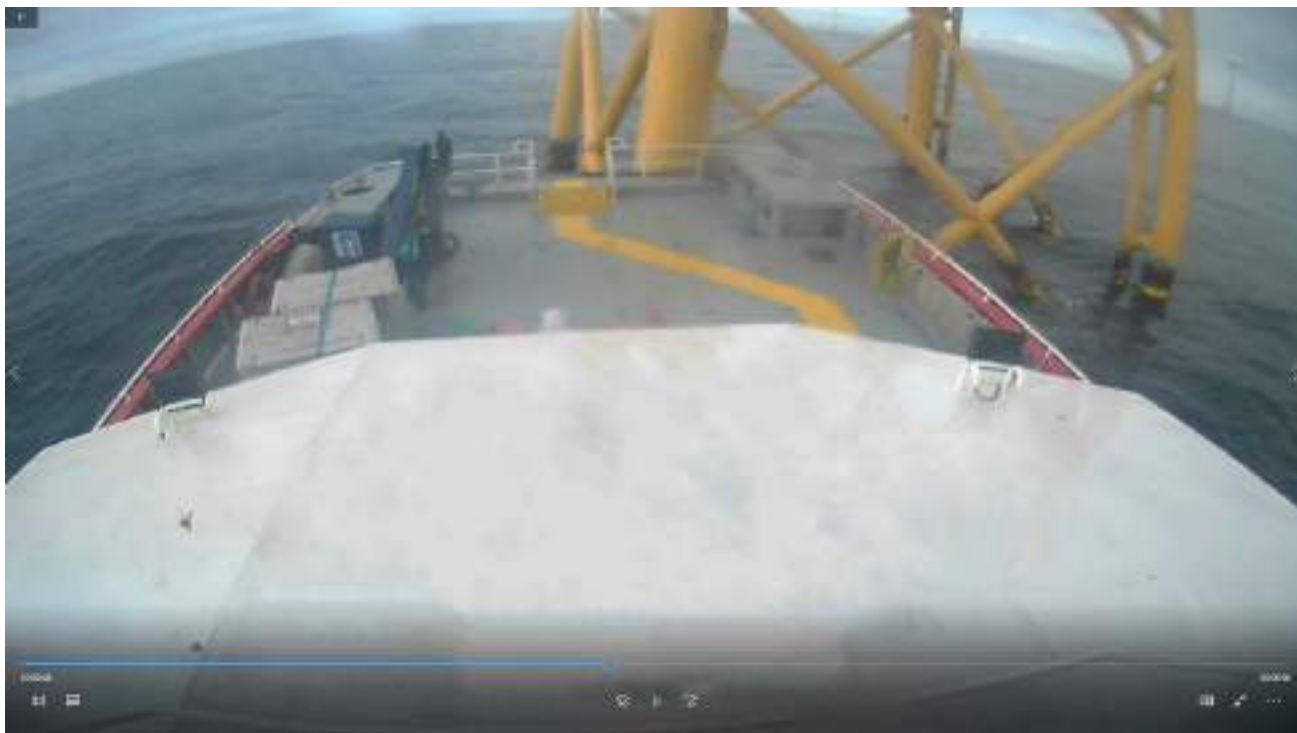
Figure 2: The moment the workboat bow collided with the wind turbine tower platform
