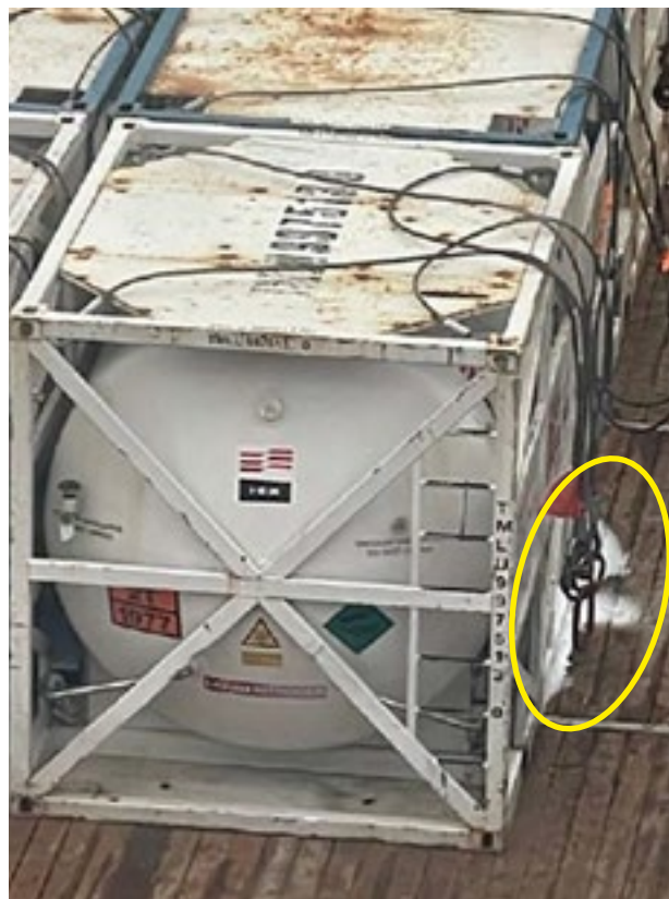
Figure 1: Icing of deck beneath nitrogen tank container
