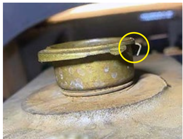
Figure 2: The bent securing lug
