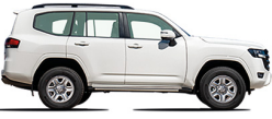
Land Cruiser 300 Station Wagon GX-R / 3.3 litre Twin Turbo Diesel V6 Automatic/Automatique/Automático 7 seater/places/plazas / 4x4 ● Code/Código: FJA300L/R-GNUAY
