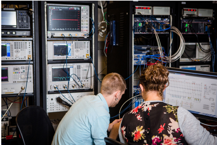
Researchers in the Engineering Quantum Systems Group, of Prof. William Oliver, setting up racks to control and measure their superconducting qubits. [Credit: Nathan Fiske]
