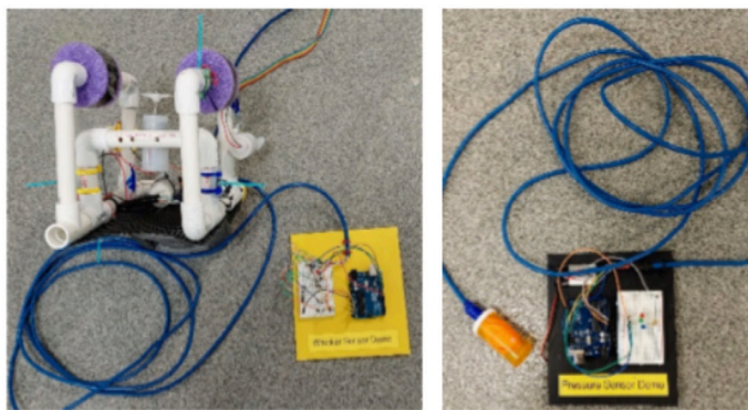
Figure 5: SeaPerch II ROV outfitted with whisker sensors (left). Educational Demo for pressure sensor (right).
