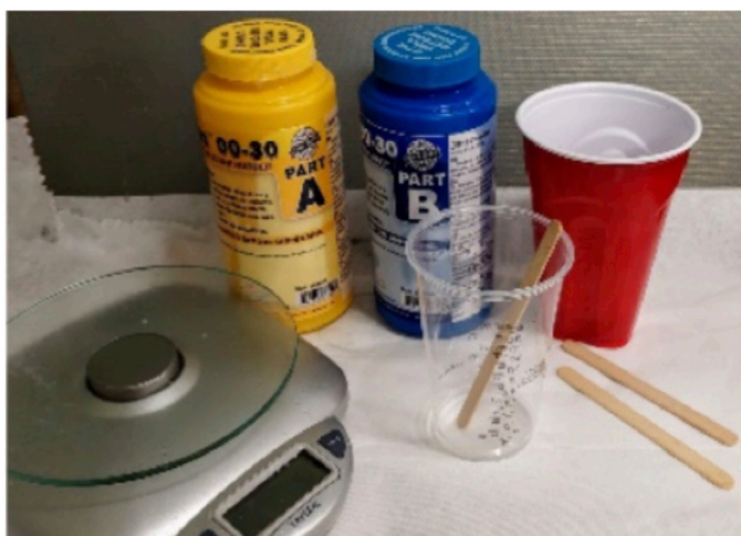
Figure 6: Materials necessary for casting with EcoFlex silicone rubber (right).
