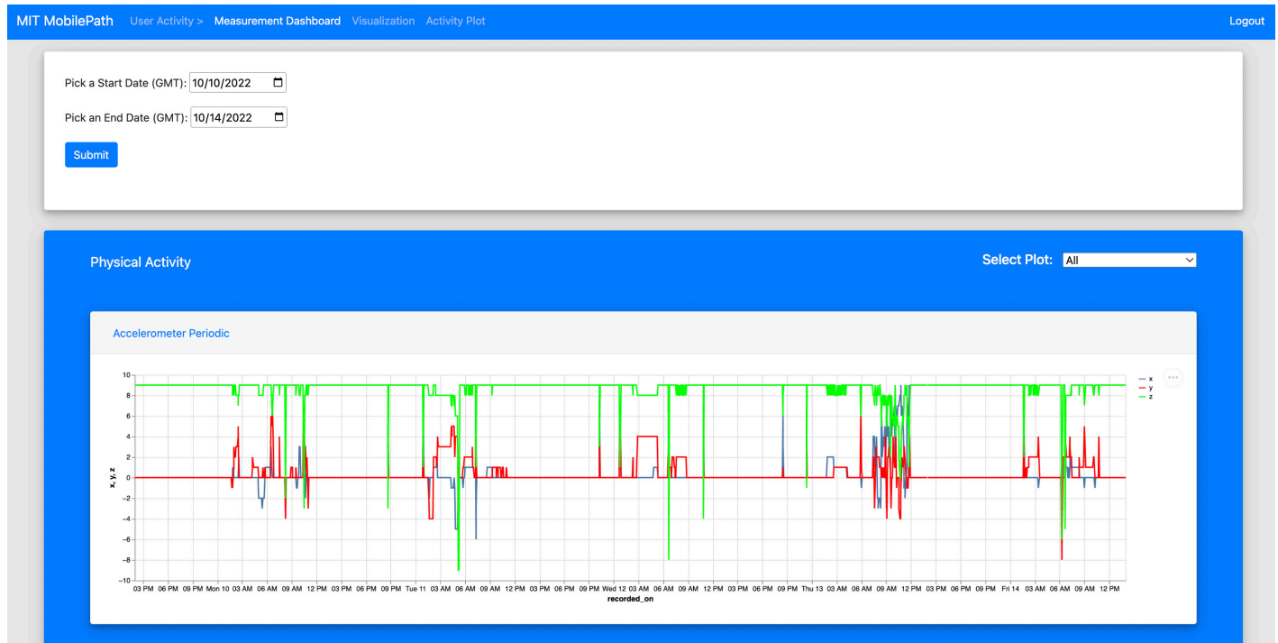
Fig. 1. MobilePath’s patient website user interface of the measurement dashboard. The measurement dashboard includes all the data collected over a specific inputted date range of that specific patient. A plot of a user’s periodic accelerometer data is displayed and graphed on MobilePath from mobile sensor data.
