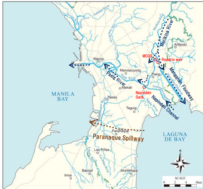
Figure 2.1.3 Hydraulic System of Laguna de Bay, Manggahan Floodway and Napindan Channel
