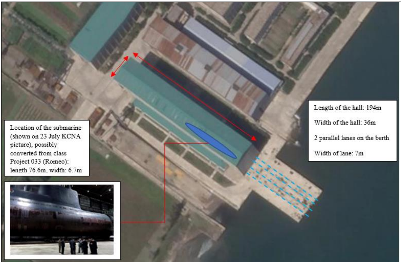
Figure 60.1: Sinpo South shipyards – new hall new berth (40° 1'20.76"N 128° 9'46.55"E) and location of the possible ballistic missile submarine (SSB) presented on the 23 July 2019 by KCNA
