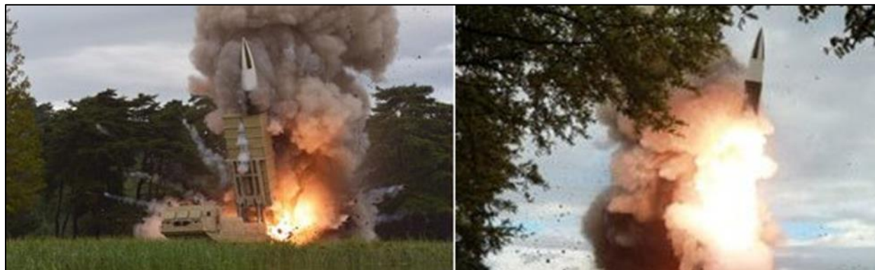
Figure 58.4.2: The two SRBMs launched on 16 August 2019 resemble the US MGM-140 ATACMS and the TEL chassis built on the DPRK Pokpung-ho battle tank chassis derived from T62 and T72 (see Figure 53.3.2)
