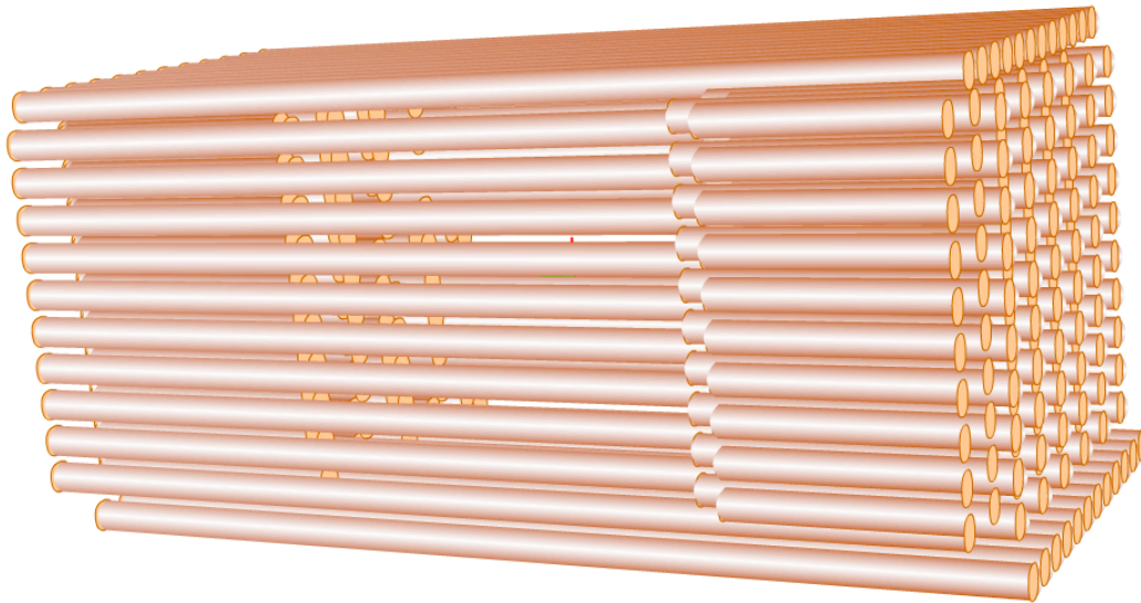
Supplementary Figure 60: Design of SS cage (square lattice arrangement), including cross-sectional view and 3D view.
