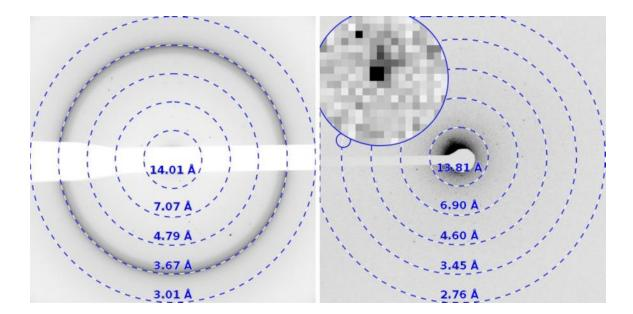
X-ray and corresponding MicroED diffraction pattern from TGF-ßm-TßRII.
