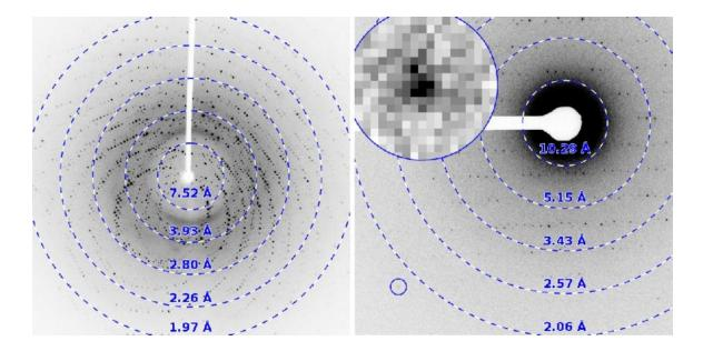
X-ray and corresponding MicroED diffraction pattern from lysozyme.
