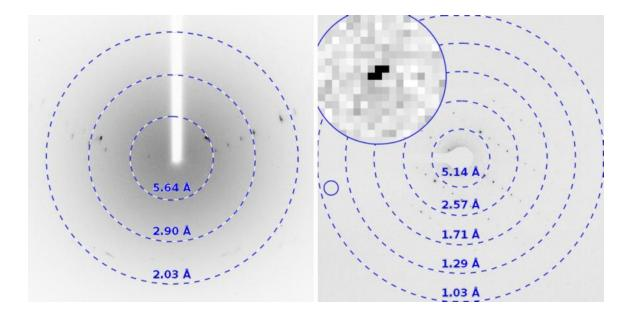
X-ray and corresponding MicroED diffraction pattern from GNNQQNY.
