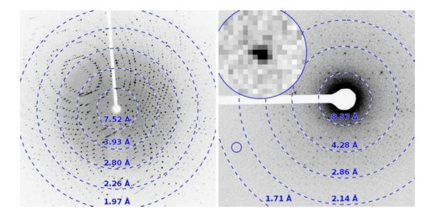
X-ray and corresponding MicroED diffraction pattern from proteinase K.
