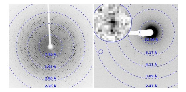
X-ray and corresponding MicroED diffraction pattern from xylanase.
