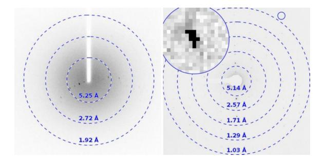
X-ray and corresponding MicroED diffraction pattern from Cd<sup>2+</sup>-NNQQNY.
