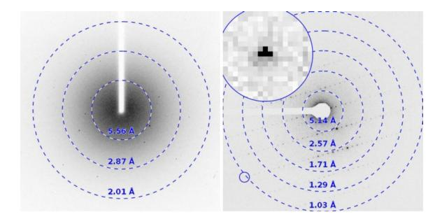
X-ray and corresponding MicroED diffraction pattern from Zn<sup>2+</sup>-NNQQNY.
