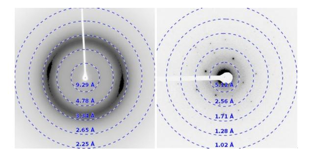
X-ray and corresponding MicroED diffraction pattern from protein tau.
