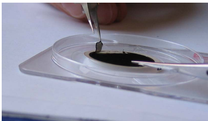
Figure S8. Photograph of NanoBud sample mat being removed from nitrocellulose filter for FE measurements.
