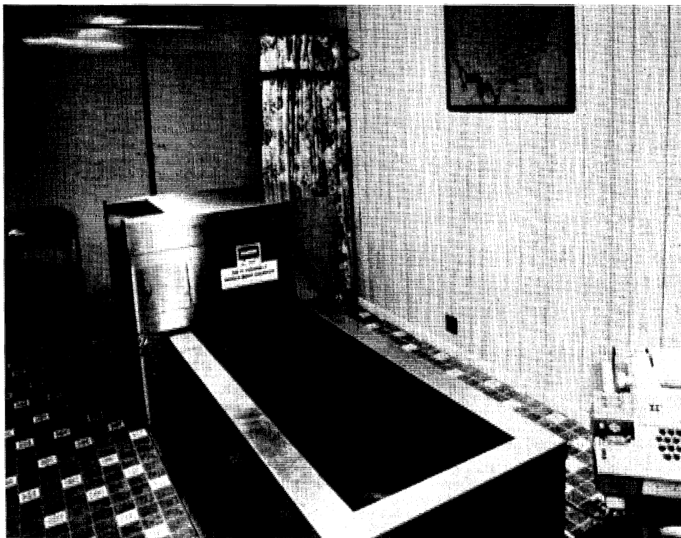
In April 1979 the NRC Office of Nuclear Reactor Regulation began a public whole body counting program at Three Mile Island using this "do-it-yourself" counter. Of more than 700 counts
