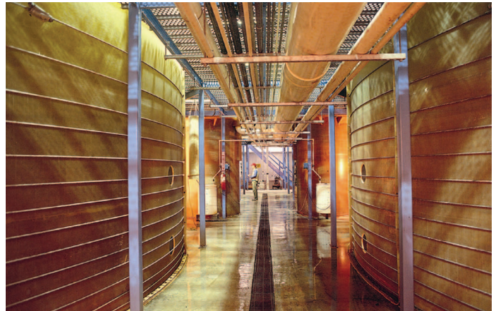
Grow-out tanks (500 t) at Australis Aquaculture's recirculating aquaculture production facility.
