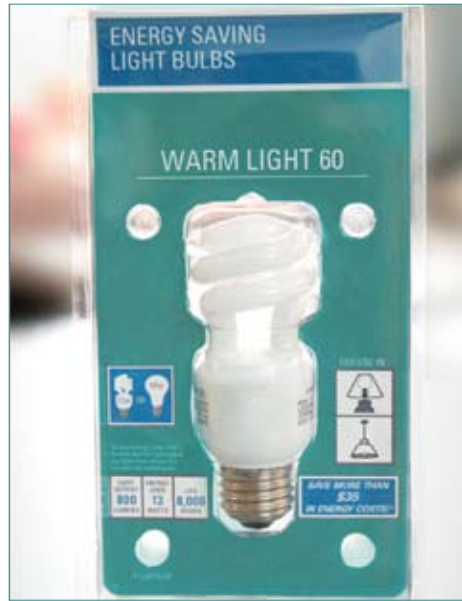
“Warm light 60” means that this CFL provides the same light as a 60-watt incandescent bulb. “Warm” indicates a color temperature between 2700-3000K.
