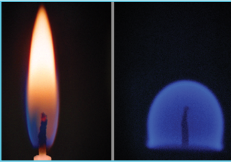
Figure 6. Left: Flames on Earth in 1-g driven by convection currents. Right: Flames in microgravity exhibiting that convection does not occur in microgravity; the hot wax from the candle does not rise; instead, the hot gas diffuses and burns when reaching a supply of oxygen. (Image Credit: NASA)
