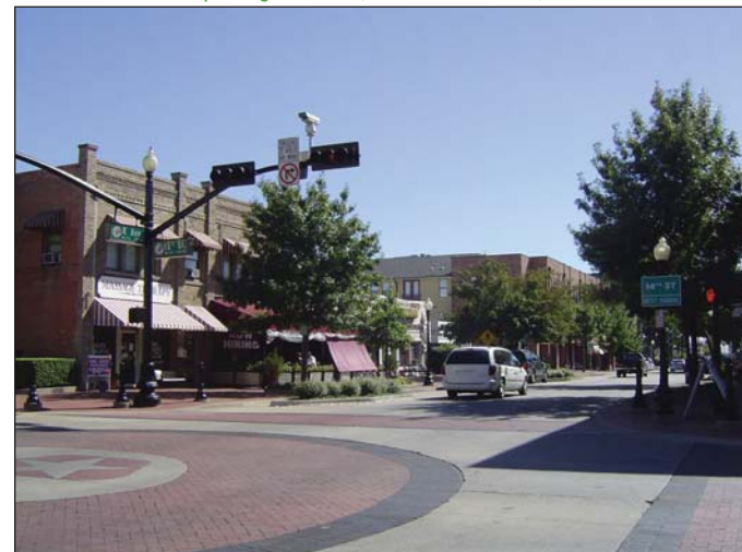
A street that uses paving textures, curb extensions, etc to calm traffic
