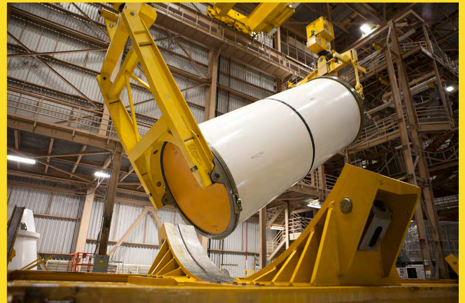
Two cranes are used in tandem to lift the first of two pathfinders, or test versions, of solid rocket booster segments for NASA's Space Launch System rocket away from a railcar inside the Rotation, Processing and Surge Facility high bay at Kennedy Space Center on Feb. 25. The booster segment will be raised into the vertical position. The Ground Systems Development and Operations Program and Jacobs Engineering, on the Test and Operations Support Contract, are conducting a series of lifts, moves and stacking operations using the booster segments, which are inert, to prepare for Exploration Mission 1, deep-space missions and the journey to Mars. The pathfinder boosters arrived at Kennedy from Orbital ATK in Utah aboard an Iowa Northern train contracted by Goodloe Transportation of Chicago. Photo credit: NASA/Ben Smegelsky
