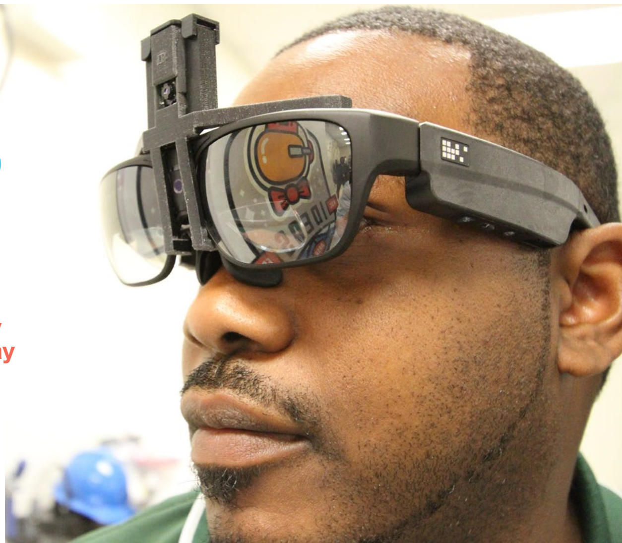
Delvin Vannorman, IDEAS software engineer, is shown modeling the Osterhout Design Group's R-7 smart glasses integrated with the IDEAS Infrared Camera and running custom NASA-developed software. Photo credit: NASA
