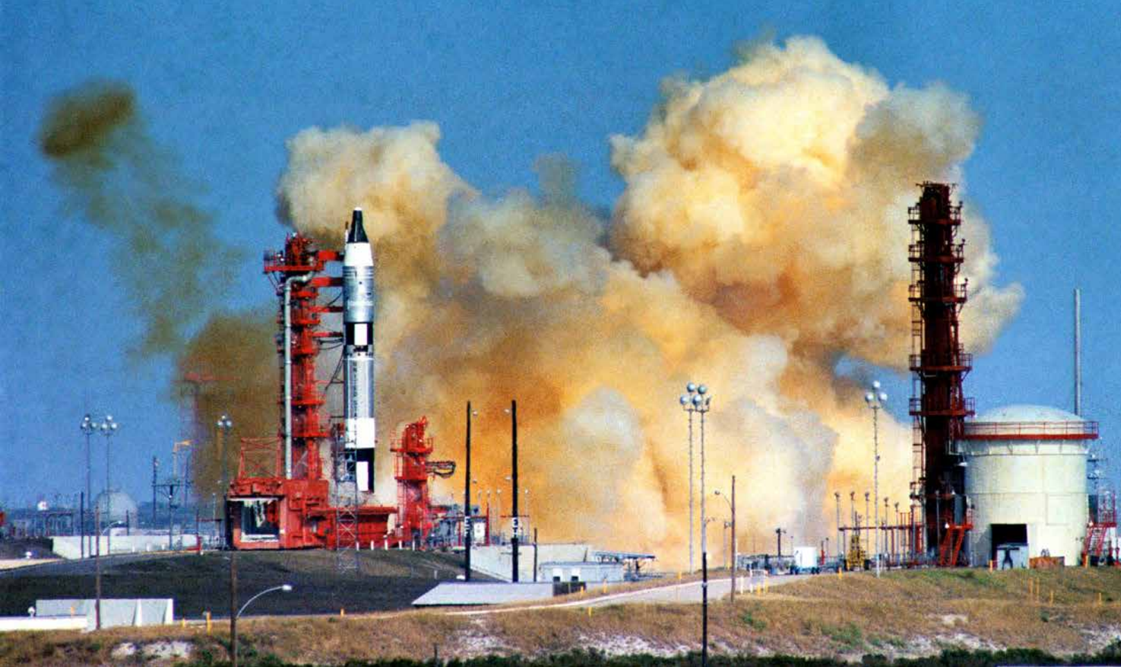
Gemini VI's Titan first stage engines shut down 1.5 seconds after ignition on Dec. 12, 1965 due to a premature release of a liftoff umbilical plug. Wally Schirra and Tom Stafford successfully launched to a rendezvous with Gemini VII three days later. Photo credit: NASA
