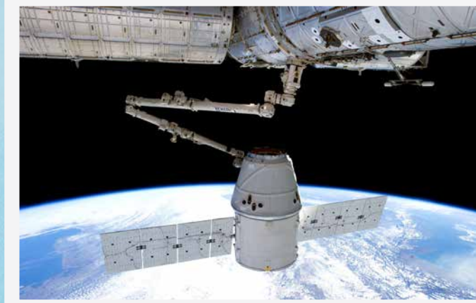
On March 3, 2013, Expedition 34 crew members aboard the International Space Station use a robotic arm to capture a SpaceX Dragon capsule delivering supplies. NASA’s commercial space program has fostered a successful partnership with American companies to resupply the station through the Commercial Resupply Services program. In the near future, a similar Dragon spacecraft will launch astronauts to low-Earth orbit as part of the Commercial Crew Program. Photo credit: NASA
