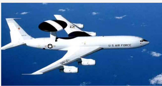
Derived from the passenger jet, the Boeing 707, the E-3 Sentry is an airborne warning and control system aircraft that provides all-weather surveillance, command, control and communications needed by commanders of U.S. and NATO air defense forces. Photo credit: U.S. Air Force photo
