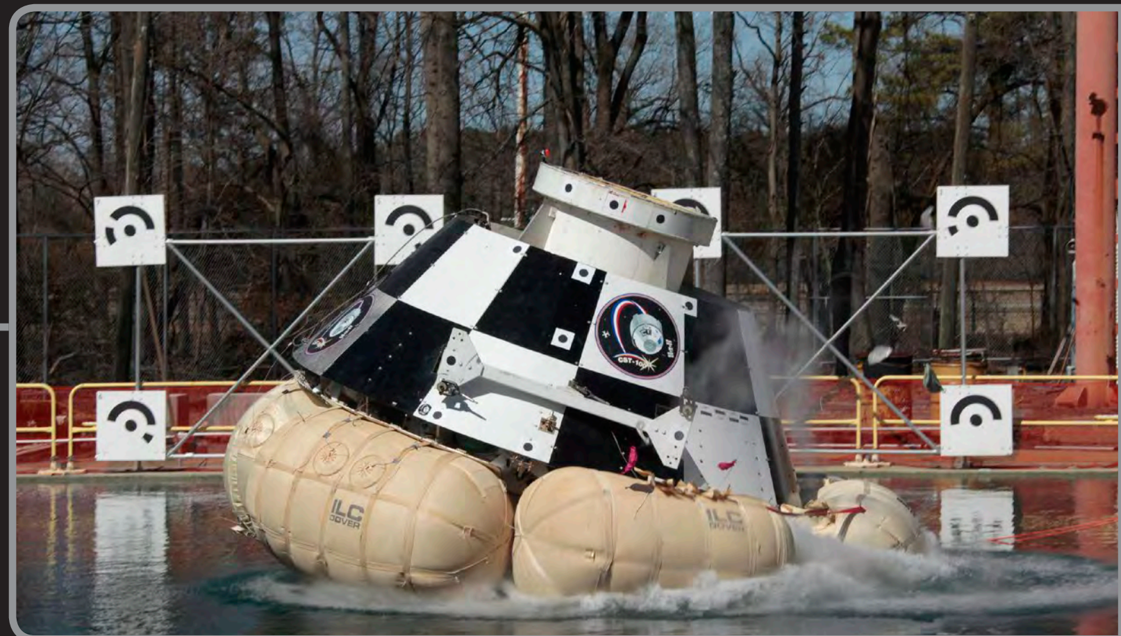
A mockup of Boeing's CST-100 Starliner splashes into a water tank at NASA's Langley Research Center in Virginia during landing system testing. Photo credit: NASA Langley
