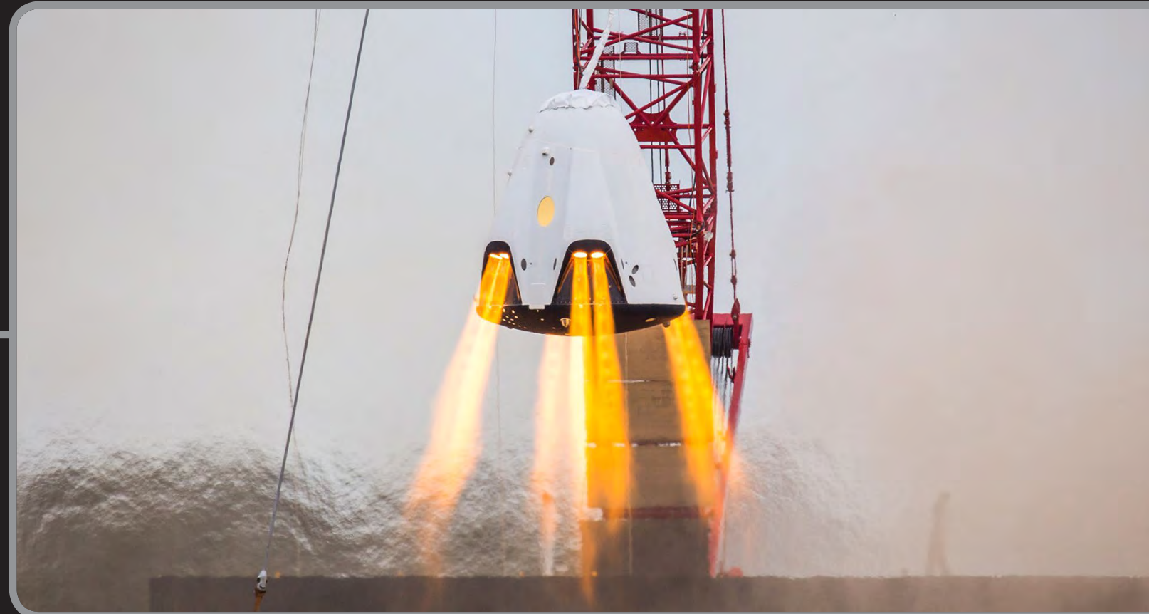
A full-size test article of a SpaceX Crew Dragon fires its eight SuperDraco engines in a development test of its ability to land with the accuracy of a helicopter using only the thrusters. Photo credit: SpaceX
