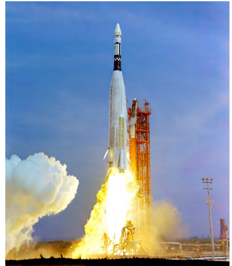
The Agena target docking spacecraft lifts off atop its Atlas rocket from Cape Kennedy's Launch Complex 14 at 3:39 p.m. EST on July 18, 1966. The Agena served as a rendezvous and docking vehicle for the Gemini X spacecraft. Photo credit: NASA
