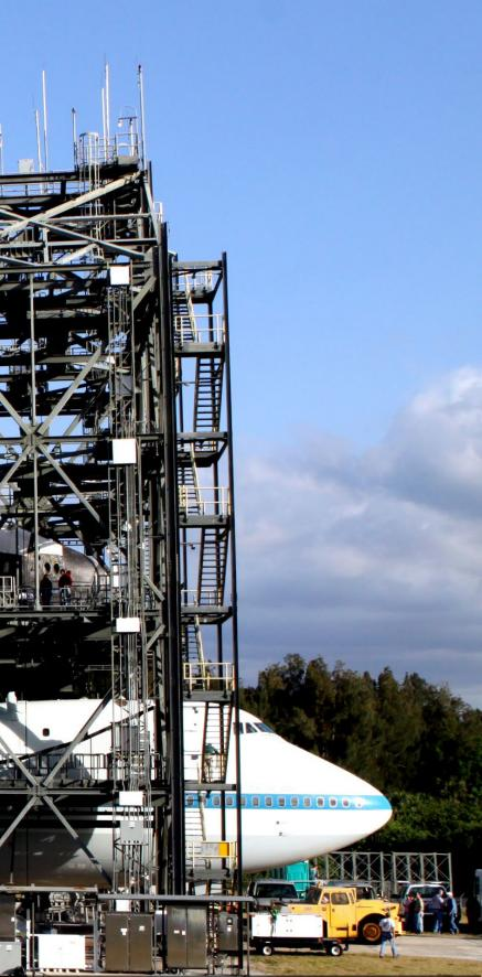
A Shuttle Carrier Aircraft is positioned beneath space shuttle Discovery in the Mate-Demate Device at the Shuttle Landing Facility at Kennedy Space Center on April 15, 2012. Discovery will be lowered and mated to the aircraft for a ferry flight to the Washington Dulles International Airport in Virginia, after which the shuttle will be on display in the Smithsonian's National Air and Space Museum Steven F. Udvar-Hazy Center. Photo credit: NASA/Kim Shiflett
