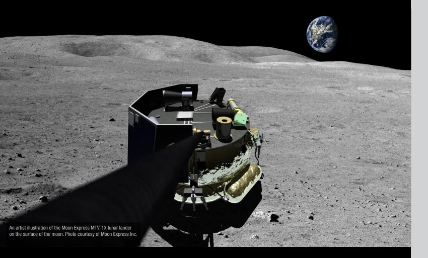
The Moon Express team has been busy since October preparing the test vehicle, called MTV-1X, for a series of tests. The compact vehicle is the size of a large coffee table. The version of this vehicle that will fly in space is a single-stage spacecraft that uses hydrogen peroxide as a primary fuel in a bi-propellant propulsion system bolstered by kerosene for its Earth departure and moon arrival burns. It's also powered by solar energy, which makes it a very green vehicle.
