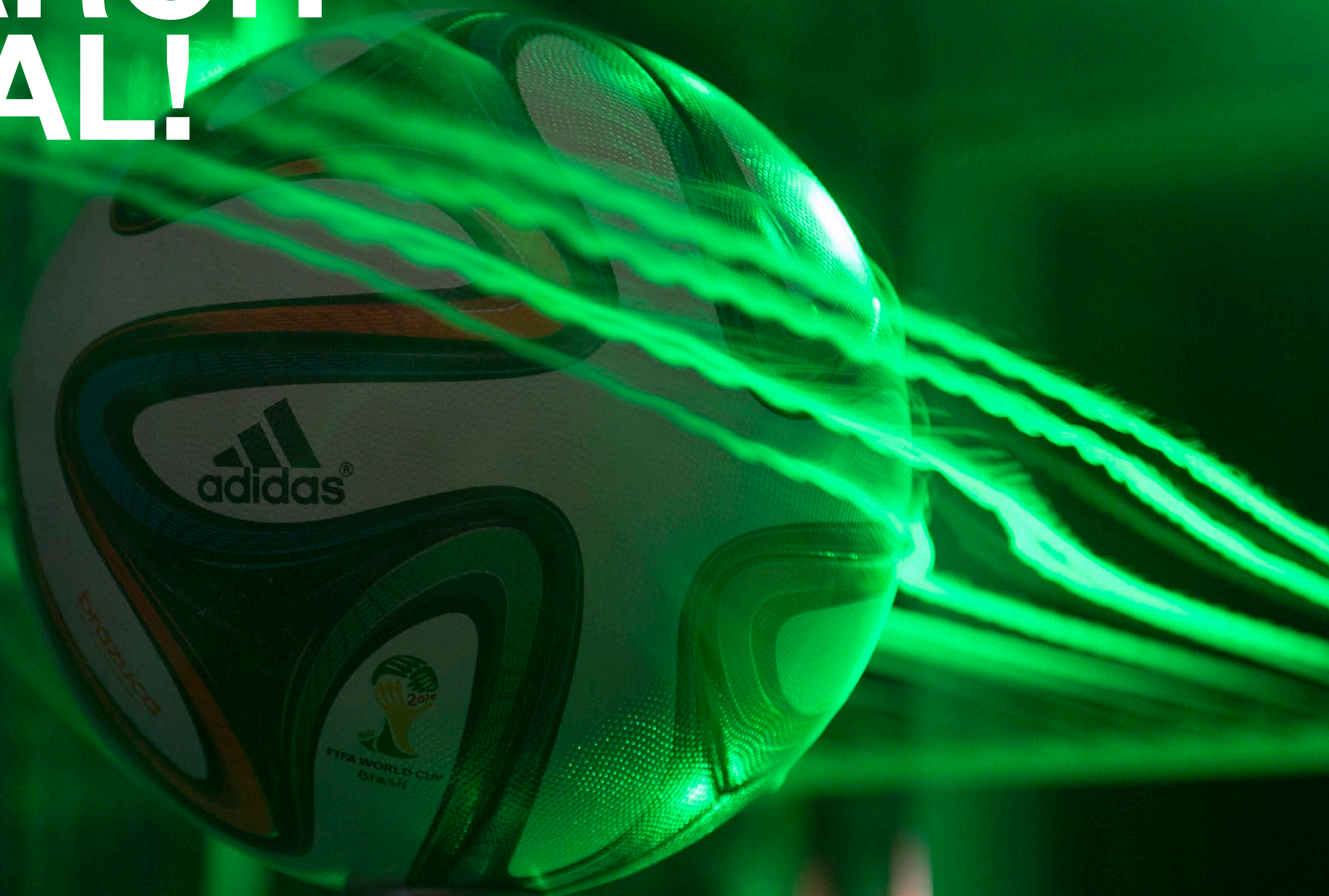
A close up of the Brazuca ball in Ames' Fluid Mechanics Laboratory's two-foot by two-foot wind tunnel. Smoke highlighted by lasers visualizes air flow around the ball. Photo credit: NASA
