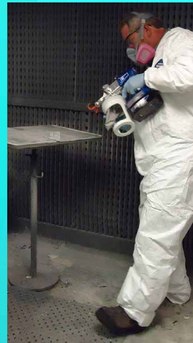
A technician sprays a protective coating on a sample panel for testing at the Beachside Atmospheric Test Facility at NASA's Kennedy Space Center. Photo credit: NASA/Jerry Curran
