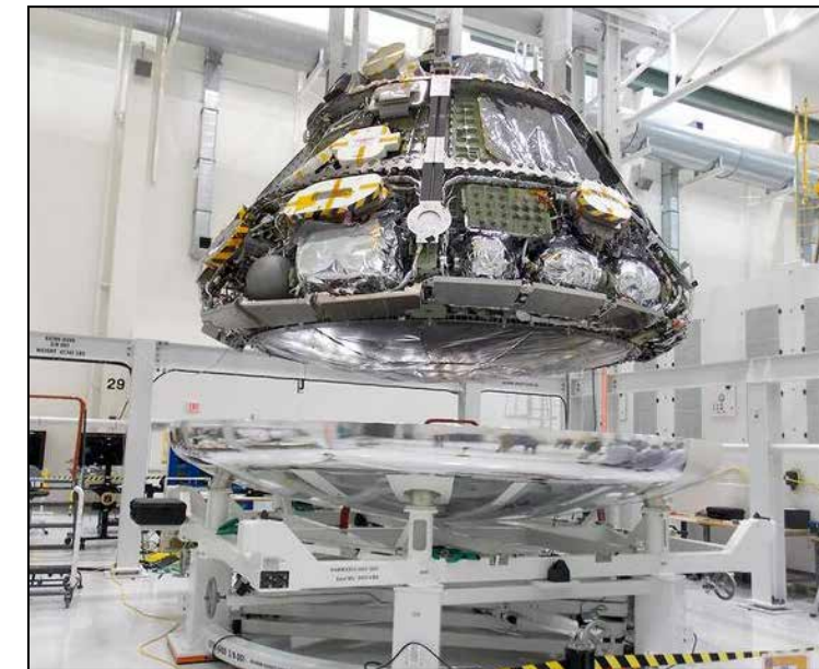
Engineers and technicians continue assembly and testing of Orion in the Kennedy Space Center's Operations and Checkout Building. On May 15, 2014, the spacecraft was suspended by a crane in position for mating operations. Photo credit: NASA
