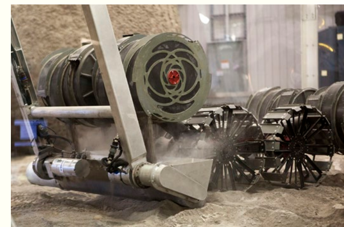
An integrated test of the MARCO POLO/Mars Pathfinder in-situ resource utilization, or ISRU, system takes place at NASA's Kennedy Space Center in Florida. Photo credit: NASA/Dimitri Gerondidakis
