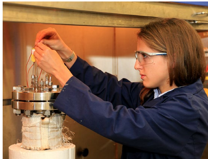
Annie Meier adjusts the trash-to-gas reactor that she is helping develop to recycle trash during deep-space missions. Unneeded materials such as scraps, wrappers, packaging and other garbage could be converted into methane gas, oxygen and water. Photo credit: NASA/Dan Casper
