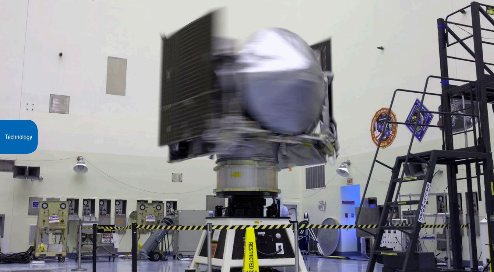
NASA's OSIRIS-Rex spacecraft rotates on a spin table during a weight and center of gravity test May 24 inside the Payload Hazardous Servicing Facility at Kennedy Space Center. The spacecraft is being prepared for its upcoming launch, targeted for Sept. 8 aboard a United Launch Alliance Atlas V rocket. Photo credit: NASA/Kim Shiflett
