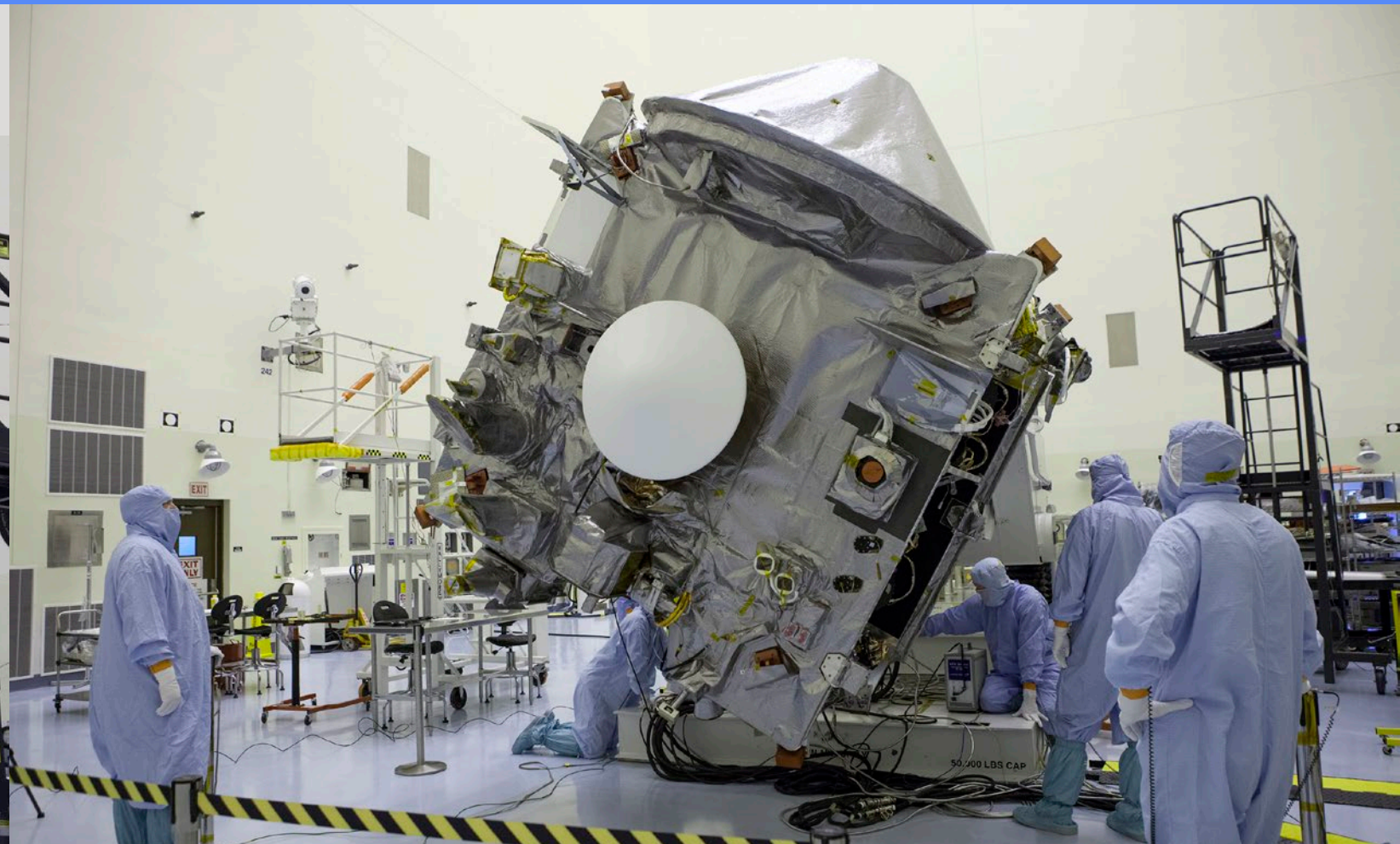
Technicians and engineers cycle the sample return capsule door July 13 in a test of NASA's OSIRIS-REx spacecraft inside the Payload Hazardous Servicing Facility at Kennedy Space Center. Photo credit: NASA/Kim Shiflett
