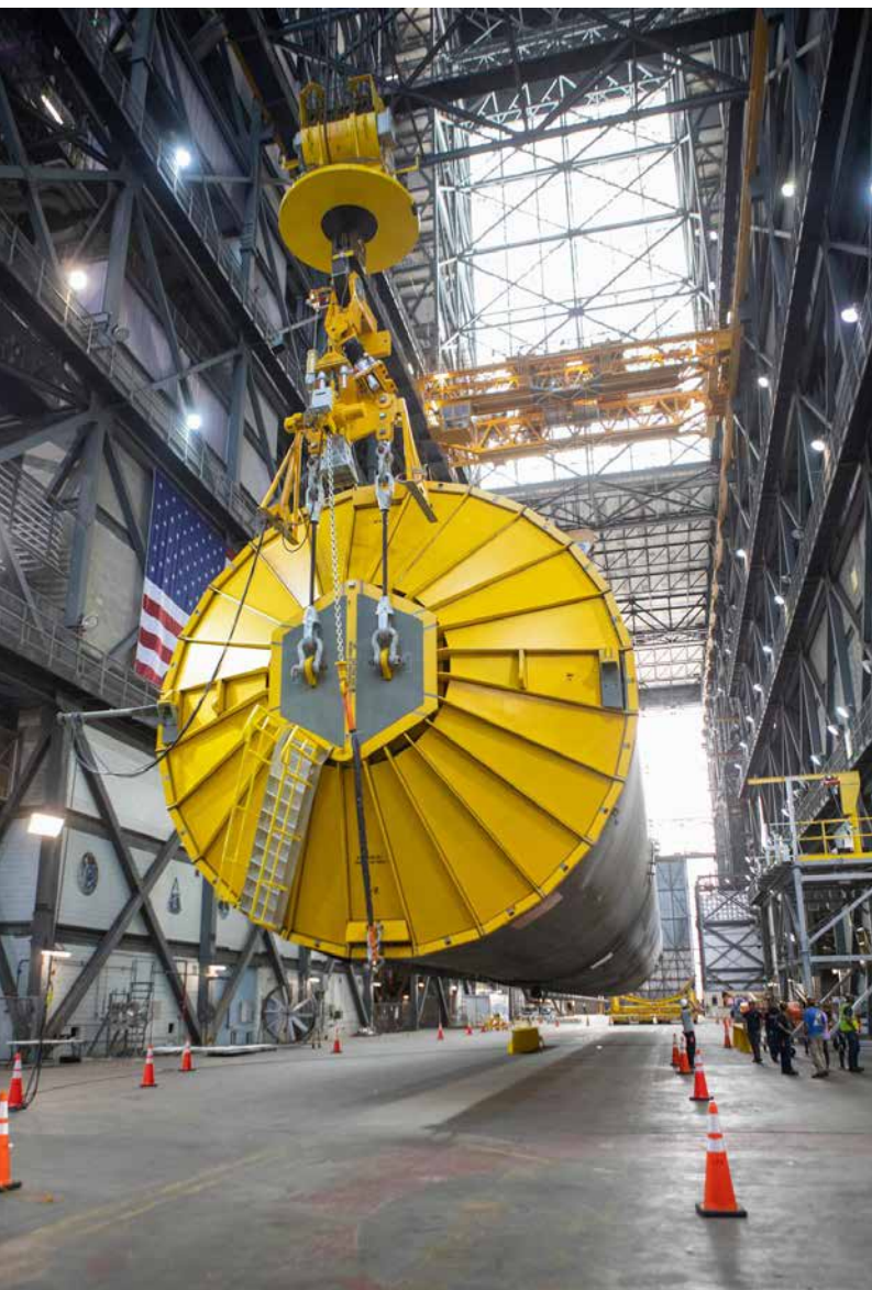
Inside the Vehicle Assembly Building at NASA's Kennedy Space Center, two cranes are used to lift the Space Launch System Core Stage pathfinder horizontally in the transfer aisle on Oct. 15, 2019. A cover, called a spider, is in view on the top of the pathfinder. A crane is attached to the spider to help lift the pathfinder. Photo credit: NASA/Ben Smegelsky
