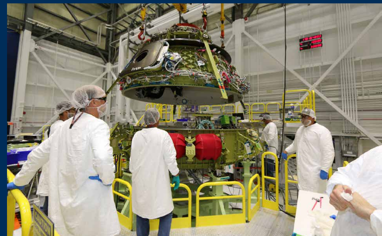
Boeing technicians meticulously lower the Starliner upper dome to the lower dome before bolting and sealing the pressure vessel. Photo credit: Boeing
