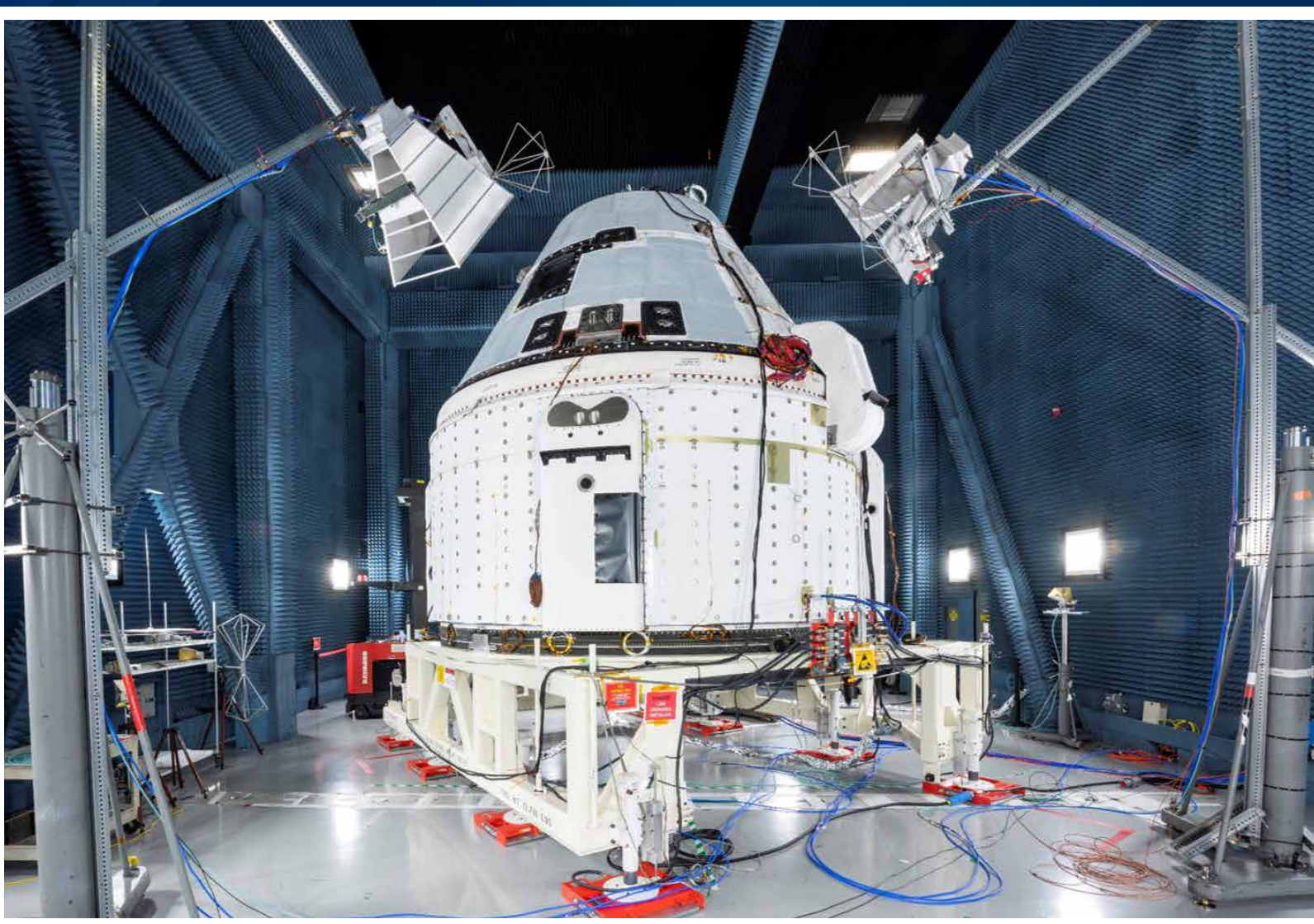
Boeing's CST-100 Starliner prepares for electromagnetic interference and electromagnetic contamination (EMI/EMC) testing in a specialized test chamber at Boeing's Space Environment Test Facilities in El Segundo, California. These tests were the final part of Starliner's environmental qualification test campaign. EMI/EMC testing ensures that Starliner's systems will function properly in the orbital radiation environment and also not interfere with other electrical systems on the International Space Station. Commercial Crew Program is working with Boeing to return human spaceflight launches to the space station from U.S. soil. Photo Credit: Boeing
