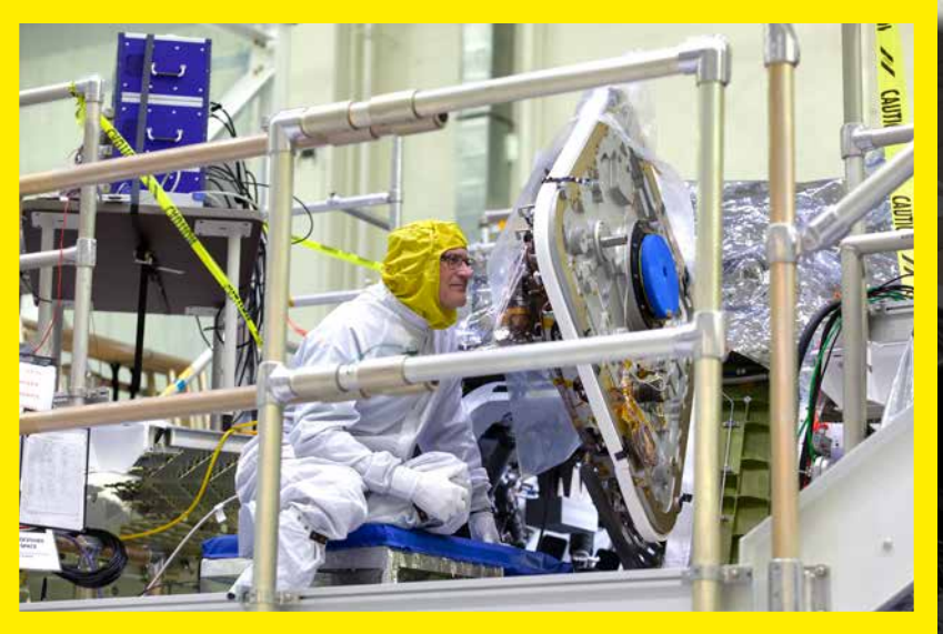
A Lockheed Martin specialist works on the hatch for the Orion crew module for Exploration Mission-1 (EM-1) on March 21, 2019, inside the Neil Armstrong Operations and Checkout Building high bay at NASA's Kennedy Space Center. Photo credit: NASA/Ben Smegelsky
