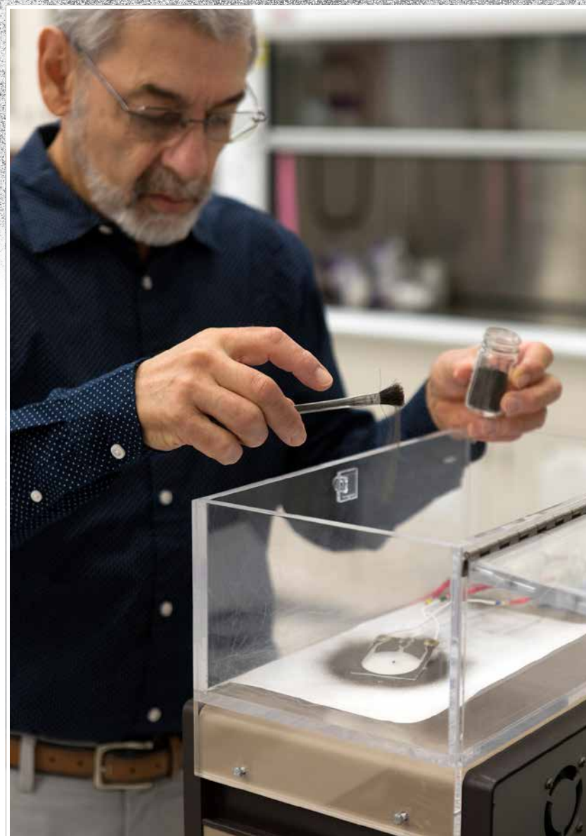
Dr. Carlos Calle has worked on the Electrostatic Dust Shield (EDS) for 15 years. He leads a team of about eight researchers striving to perfect the technology that uses dynamic electric fields to remove dust from surfaces. Calle is hopeful that the EDS will play a major role in NASA's plans to send humans back to the Moon and on to Mars. Photo credit: NASA
